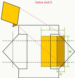
3. Internal two-part sleeve (four components). Two sheets of varying length are glued on the pocket and two sheets of varying length are glued on top.
