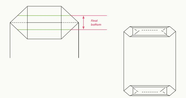
2. Stepped-end tubes have a more complex construction, but are more efficient with respect to material savings, flat-bottomed surface and reinforced bottom. Due to the stepped material edges, it is possible to glue each ply together in the overlapping area of the bottom flap. The bottom corners become tighter as the restoring force of the bottom fold decreases.
