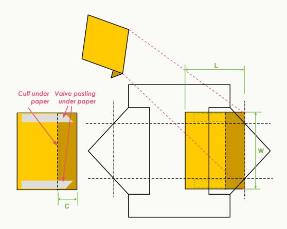
2. Double-sheet valve. The first sheet is glued on the pocket and the second sheet is glued on top. This increases the tightness, as the paper sheet overlaps the pocket depth.
